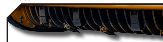
Fixed tooth with tip in tungsten
