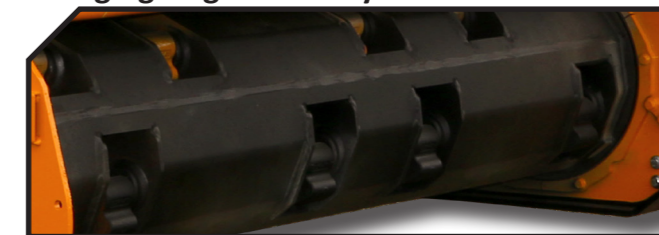
Fixed tooth with tip in tungsten
