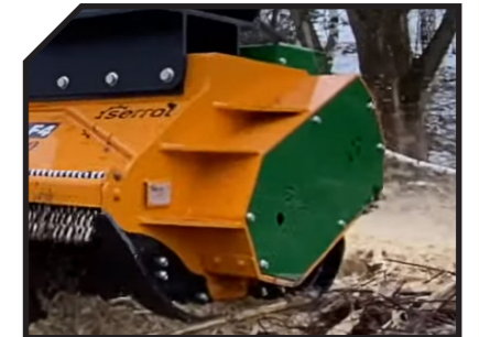
Fixed tooth with tip in tungsten
