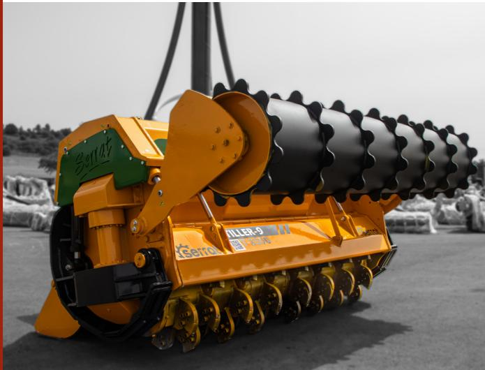
Soil preparation machine up to a depth of 700 mm, for tractors between 400 - 700 HP. Transforms forest land, with stumps and rocks, in land for cultivation avoiding accidents in later processes.
