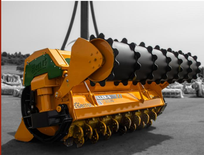
Soil preparation machine up to a depth of 600 mm, for tractors between 400 - 500 HP. Transforms forest land, with stumps and rocks, in land for cultivation avoiding accidents in later processes.
