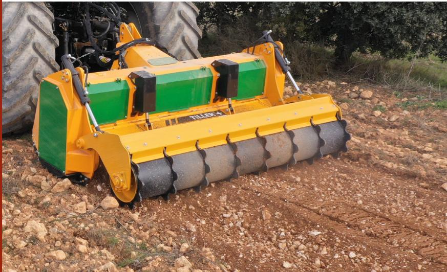
Soil preparation machine up to a depth of 300 mm, for tractors between 250 - 300 HP. Transforms forest land, with stumps and rocks, in land for cultivation avoiding accidents in later processes.
