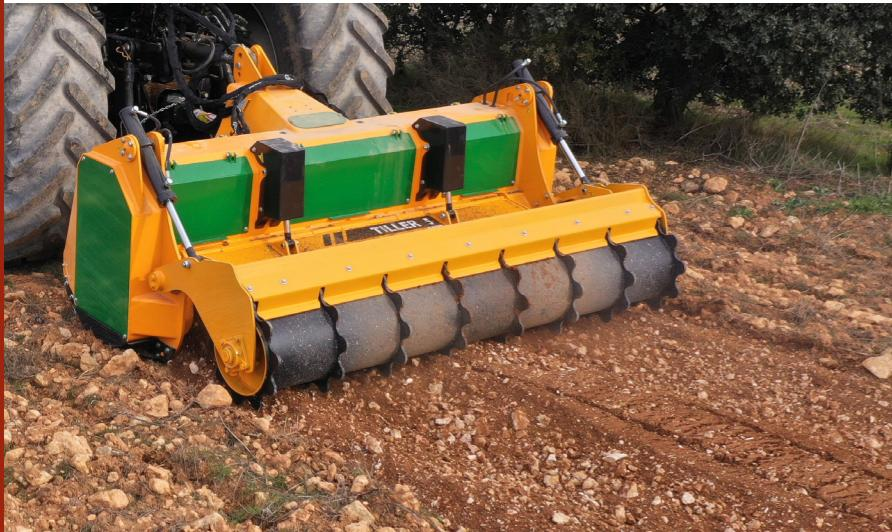
Soil preparation machine up to a depth of 200 mm, for tractors between 150 - 200 HP. Transforms forest land, with stumps and rocks, in land for cultivation avoiding accidents in later processes.
