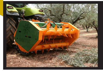
Mulcher with reversible hydraulic feeder for tractors between 220-350 HP, ideal for wood until 250 mm of diameter.
