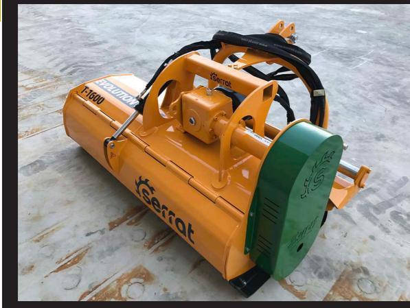
Mulcher designed for tractors between 60 HP to 120 HP for the maintenance of vegetable mantle and for the elimination of remains of pruning up to 80 mm.
