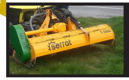
Mulcher designed for tractors between 30 HP to 80 HP for the maintenance of vegetable mantle and for the elimination of remains of pruning up to 50 mm.
