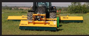
Heavy-duty high body mulcher conceived for very large farms and agricultural contractors. Robust machine designed for very intensive mulching, intended for mulching grass in park maintenance, straw, maize stalks, and on fallow land. Composition for big tractors reaching a working width of 10 meters with a front machine
