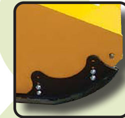
▶ Front adjustable skid shoes only for straight side
